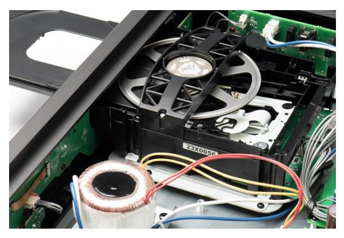
There aren't a lot of CD drive mechanisms being manufactured these days, so the fact that TEAC builds its own, and a decidedly unique one at that, is interesting. The fact that a version of the VRDS mechanism is also used in the \$25,000 Esoteric K-01XD SE SACD transport also hints at a noteworthy pedigree.
